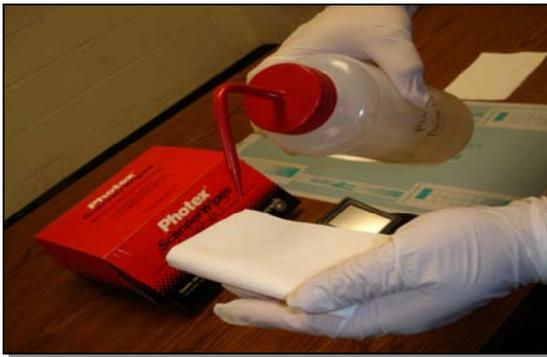
**Figure 3 Photex Wipes being dampened with Plate Developer**
